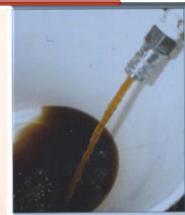
The manganese in the treated water oxidized in the distribution system and resulted in black-brown water at the tap.
